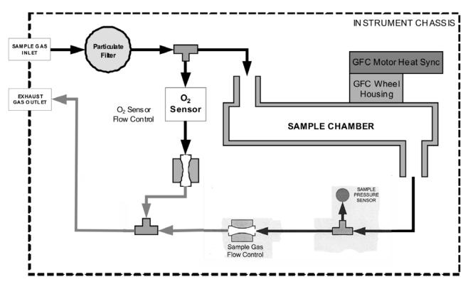
Figure 12-11: GFC7001T/GFC7001TM – Internal Pneumatics with O₂ Sensor Option 65A
